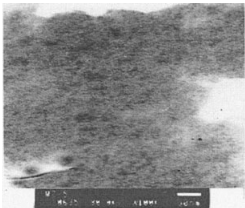
Figure 2 A transmission electron micrograph of the epoxy-silica hybrid. Scale bar = 50 nm.
